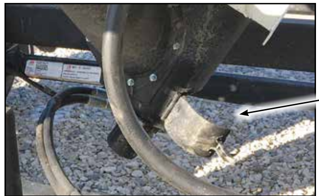
Fig 38 - Bottom clean-out access door
