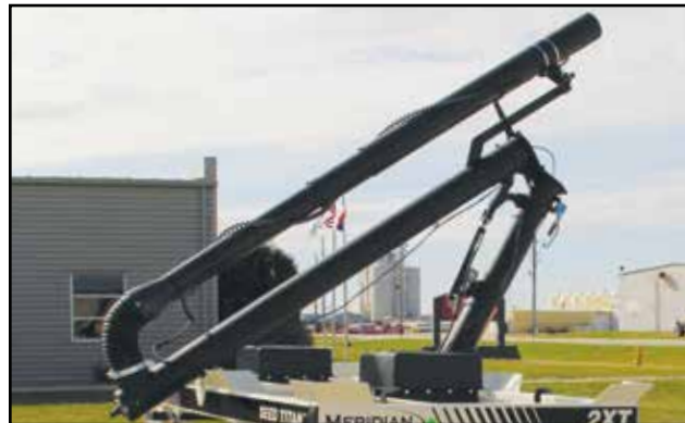
Fig 36 - Auger tube in transport position
