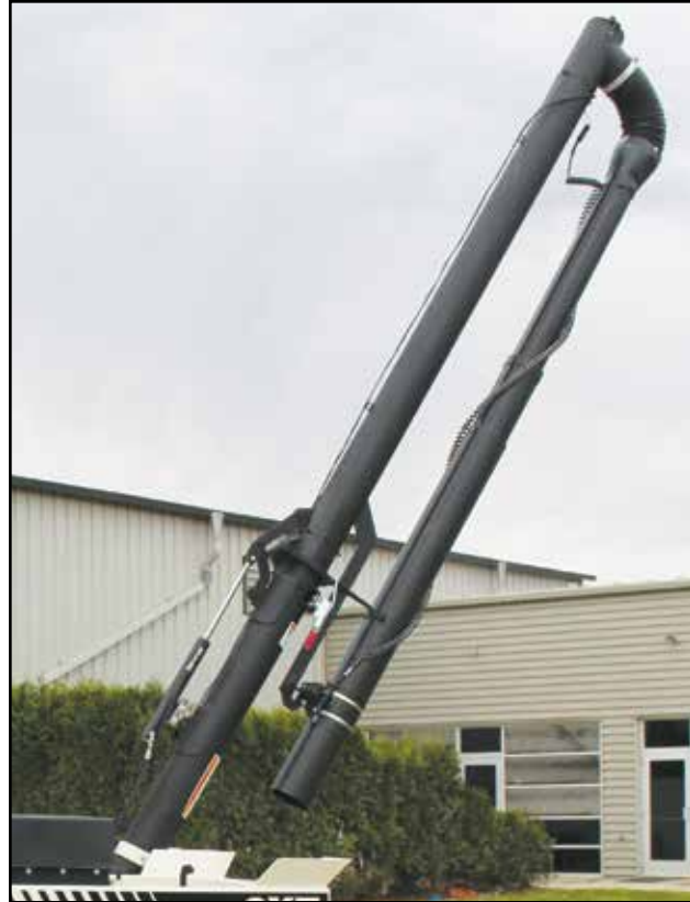
Fig 35 - Auger tube and delivery spout
