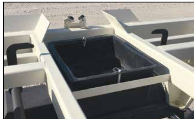
Fig 27 - Hopper cover in storage
