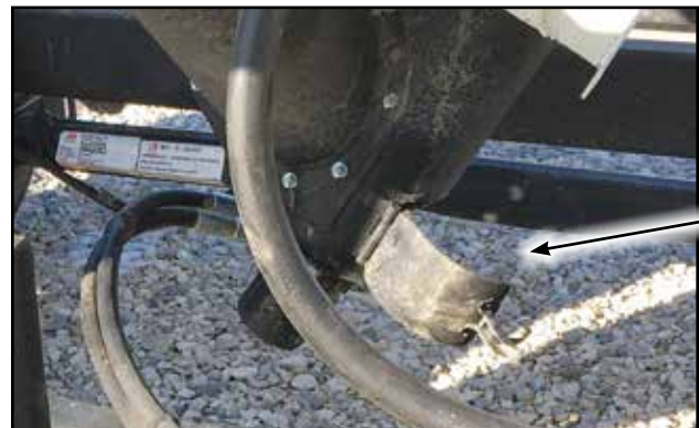
Fig 10 - Bottom clean-out access
