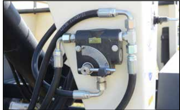
Fig 7 - Flow control valve
