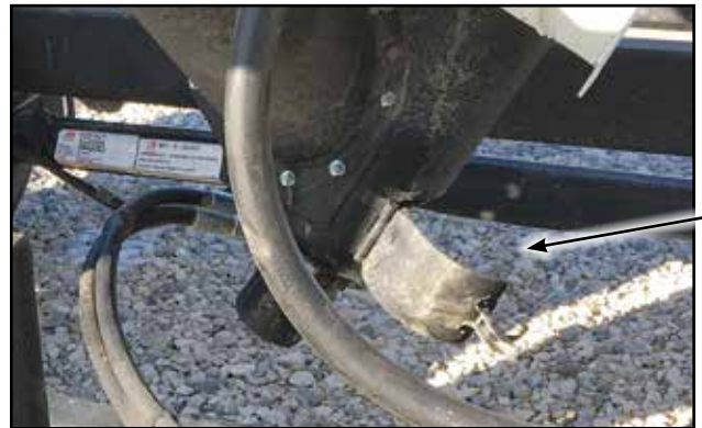
Fig 47 - Bottom clean-out access door
