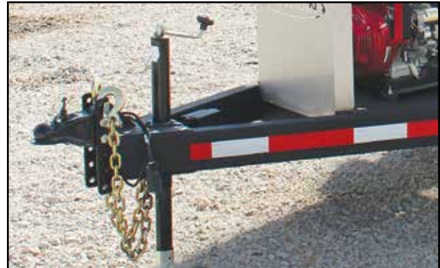
Fig 23 - Trailer jack and hitch receiver
