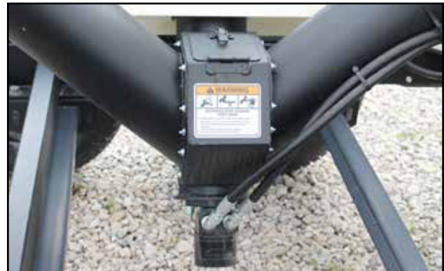
Fig 9 - Hydraulic auger motor and auger clean-out access
