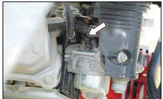
Fig 43 - Engine speed setscrew
