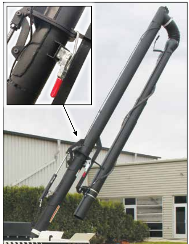
Fig 13 - Auger tube in place, ready for operation
