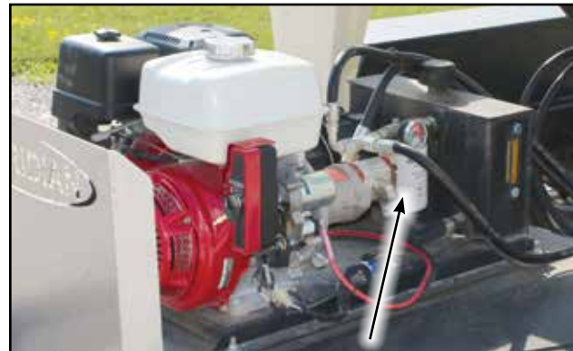
Fig 44 - Hydraulic oil filter
