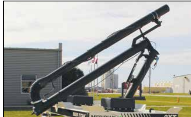
Fig 30 - Auger tube in transport position
