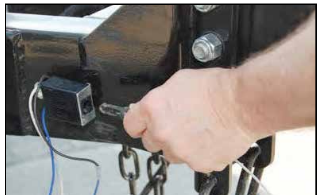
Fig 21 - Test Break-Away pin
