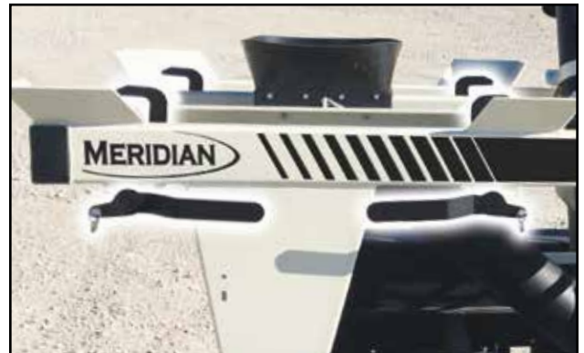
Fig 28 - Seed box lock-down handles and latches
