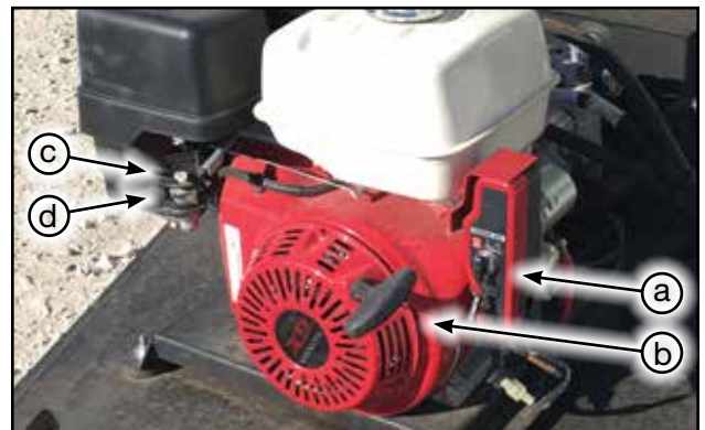
Fig 5 - Gas engine controls
