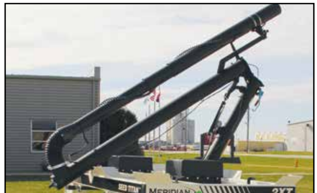
Fig 12 - Auger tube folded for transport and storage
