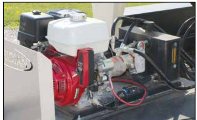
Fig 6 - Gas engine, hyd pump and oil reservoir
