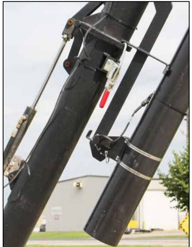
Fig 34 - Tube clamp and delivery spout
