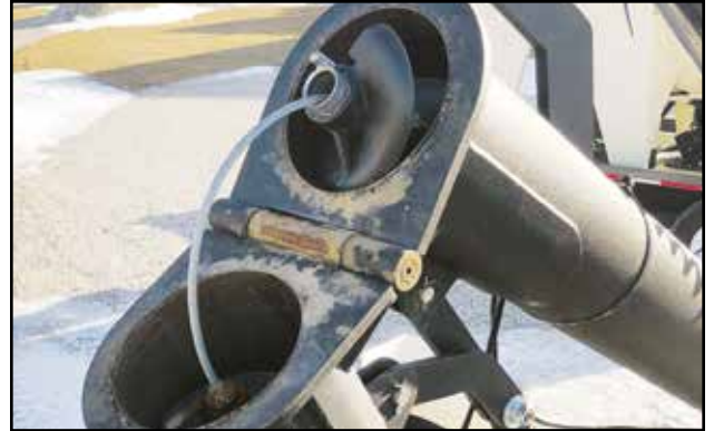
Fig 32 - Auger drive coupling
